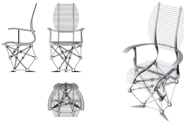
Figure 4. Tensegrity chair designed by Nebojša Vortovšek at the Spatial Structures course
