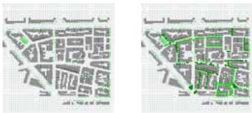
Figure 14. Digital models of the project site for microclimate simulations (envimet input file) (a) before interventions and (b) after interventions source: Bioclimatic Study, Directorate of Urban Planning and Architectural Studies, Municipality of Thessaloniki
