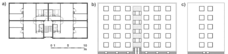
Figure 5: a) Typical floor plan; b) side façade; c) longitudinal facade of the selected multifamily housing building
