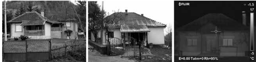
Figure 7. House type 1 and the thermo-vision photo of the construction (photo Ksenija Bunjak).
