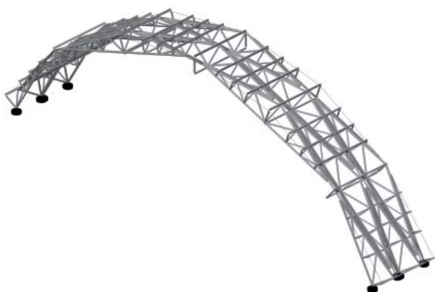
Figure 5. Isometric view of the prototype of folded construction
