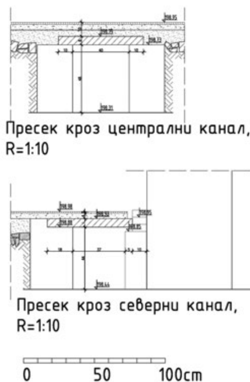
Fig. 11. Reconstruction of the cross-section of central and east channel of the heating system (drawing I. Bjelić)
