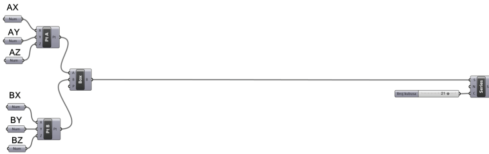
Figure, 13 - Grasshopper's segment for six numerical lists cubic element's corner management
