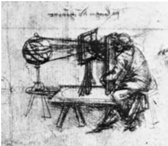
Fig. 2 Leonard da Vinci, Man using a transparent plane to draw an armillary sphere (c. 1510)
