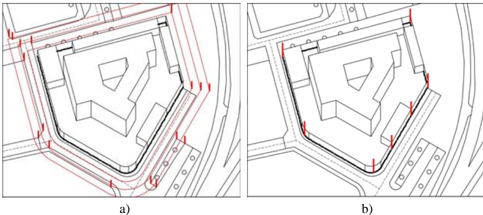
Fig. 6 Security. a) Security perimeter extending beyond the plot, CCTV cameras in public spaces. b) Security perimeter within the boundaries, checkpoint CCTV surveillance.
