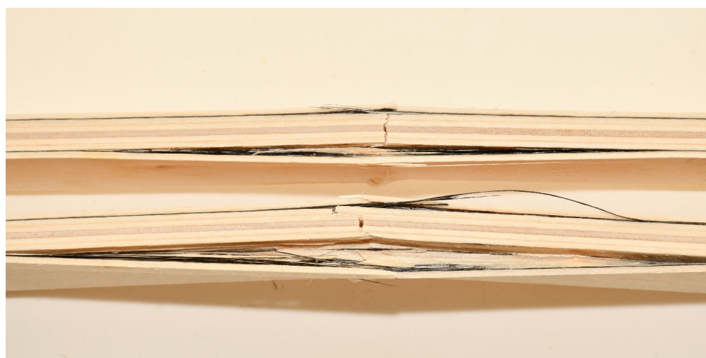
Figure 11. Substrate failure sampling for EK1OP2-SE3 and EK1OP3-SE3.
