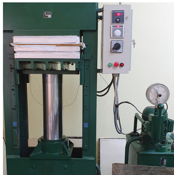
Figure 2. Process of pressing LVL panels in a laboratory press.
