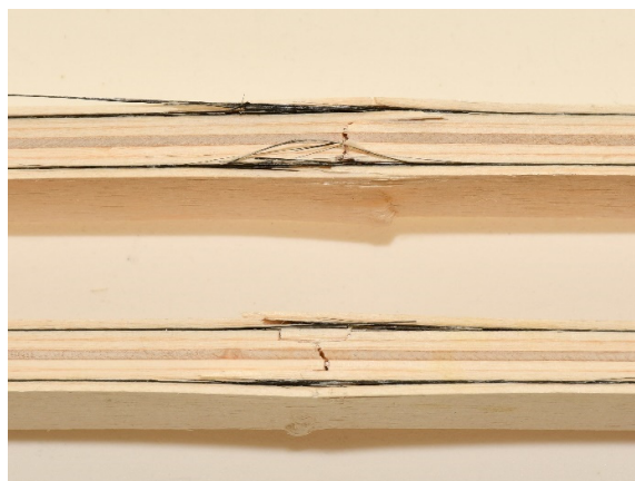
Figure 10. EK1 samples failure from edgewise bending: wood layer cracking and fiber tearing.
