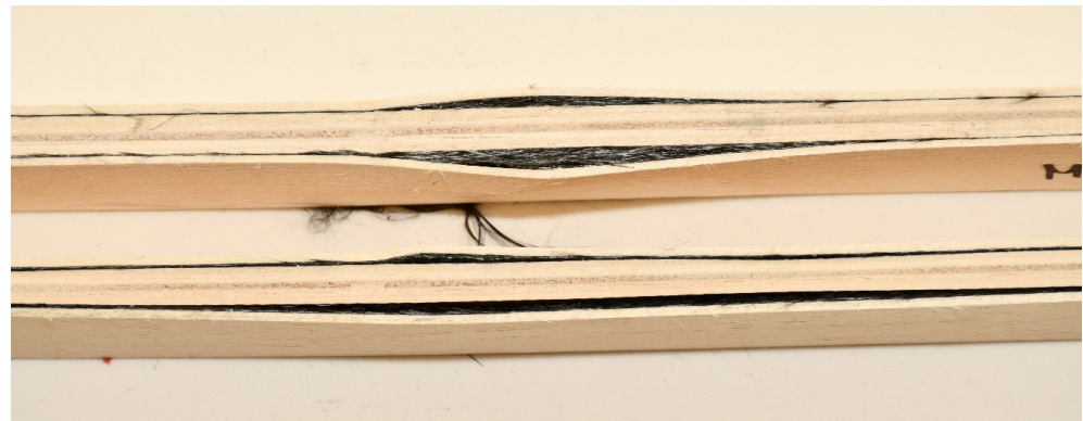
Figure 18. Delamination in the FRP-FRP layer in the test samples from MK3 panels after testing.
