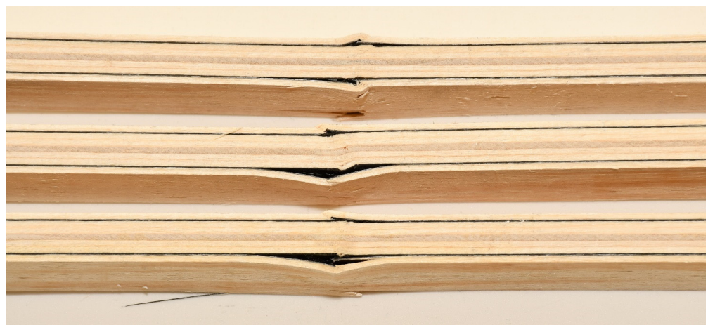
Figure 12. Failure of test samples EK3 in the pressure zone, crushing of fibers, and delamination in the FRP-FRP layer.
