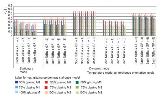
Figure 8. F<sub>x</sub> values for three analyzed models with respect to orientation and air exchange rate (for color image see journal web site)
