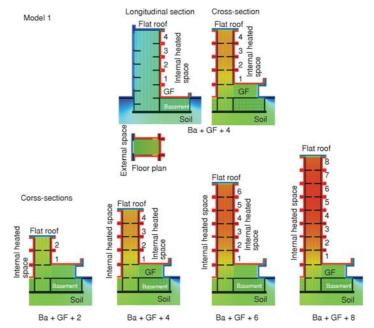
Figure 3. Temperature distribution pattern along the Ba + GF + 4 high model M1 staircase area (top) and variations in temperature distribution due to the change of building height (bottom) (for color image see journal web site)
