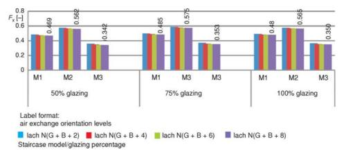
Figure 6.  $F_x$  values for three analyzed models with respect to the glazing percentage (dynamic temperature mode: 1 exchange per hour and northern orientation) (for color image see journal web site)
