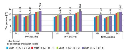
Figure 4. Average temperature values for three analyzed models with respect to the glazing percentage (stationary temperature mode) (for color image see journal web site)
