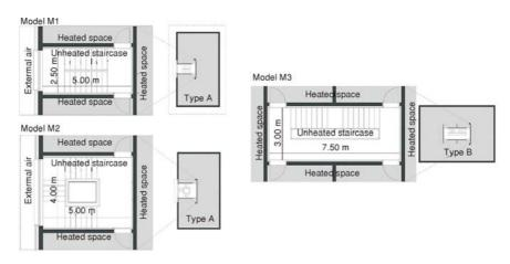
Figure 2. Geometry and disposition within a floor plan of model staircases
