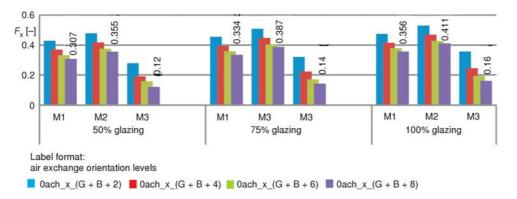
Figure 5.  $F_x$  values for three analyzed models with respect to the glazing percentage (stationary temperature mode) (for color image see journal web site)
