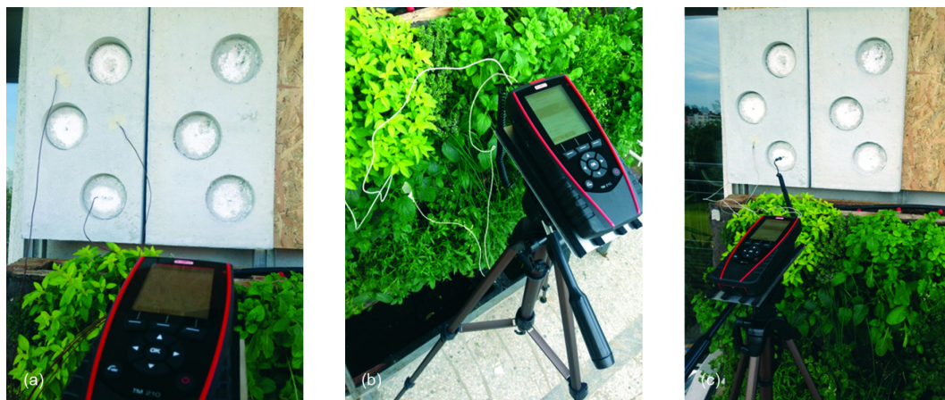
Figure 4. Measuring contact temperatures (photos by authors)
