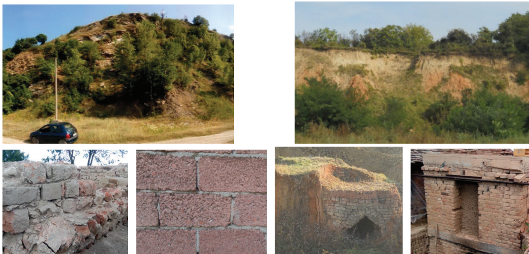
Figure 2: Ram stone quarry, crvenka quarry, brick kilns from Viminacium , brick kiln in a present day village near Viminacium, Viminacium wall made of crvenka , modern blocks made with crvenka (photos: E. Nikolić)
