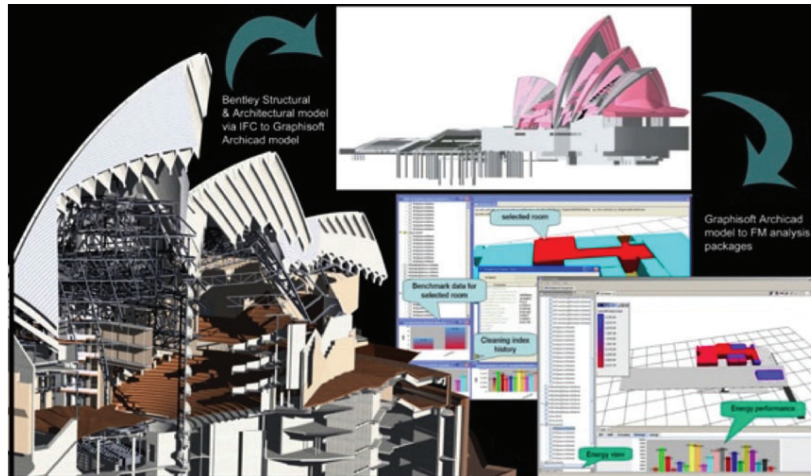
Figure 7 Sydney Opera House – An examination of interoperability between BIM and FM applications (source of illustration Mitchell and Schevers. 2006, pp. ix)
