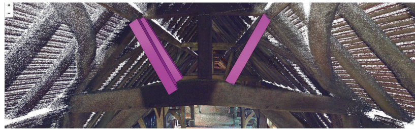
Figure 4 , Harmondsworth Barn – the hybrid model combining a scanned cloud of points with modelled intelligent objects, available at http://bim4h.org/hybrid-panos/1.html
