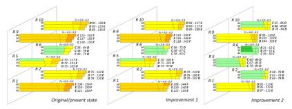
Figure 5: Specific annual energy for heating  $Q_{h.an}$  [kWh/m<sup>2</sup>] and energy class of rooms for south orientation of themain facade
