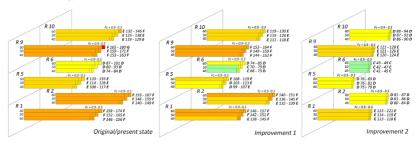
Figure 4: Specific annual energy for heating  $Q_{h.an}$  [kWh/m<sup>2</sup>] and energy class of rooms for north orientation of themain facade
