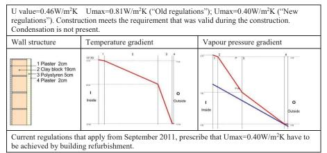
Laying of thermal insulation on external wall surface enables thermal bridges break and provides existing external massive wall to be converted into energy rational structure consisting of three layers: existing solid wall as thermal storage layer, thermal insulation and external protective and final layer as re-cladding (Krstic-Furundzic and Rajcic, 2000). Rehabilitation measure included creation of the second and third layer.
