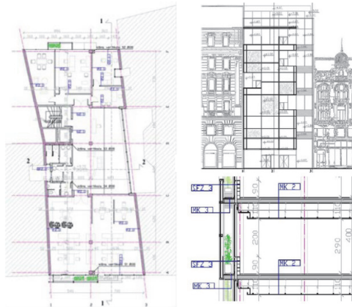
Figure 7. Plan of a typical floor, elevation and cross-section of the street facade of Model 2
