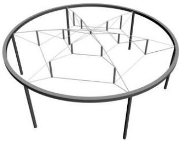
Figure 13a - Non-triangulated tensegrity type cable dome model
