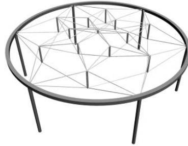
Figure 13b - Triangulated tensegrity type cable dome model
