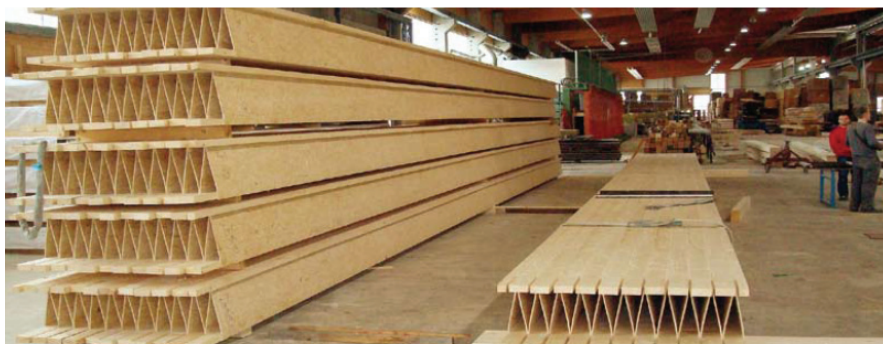
Fig. 5. Mezzanine ceiling called "Kielsteg"[26]
