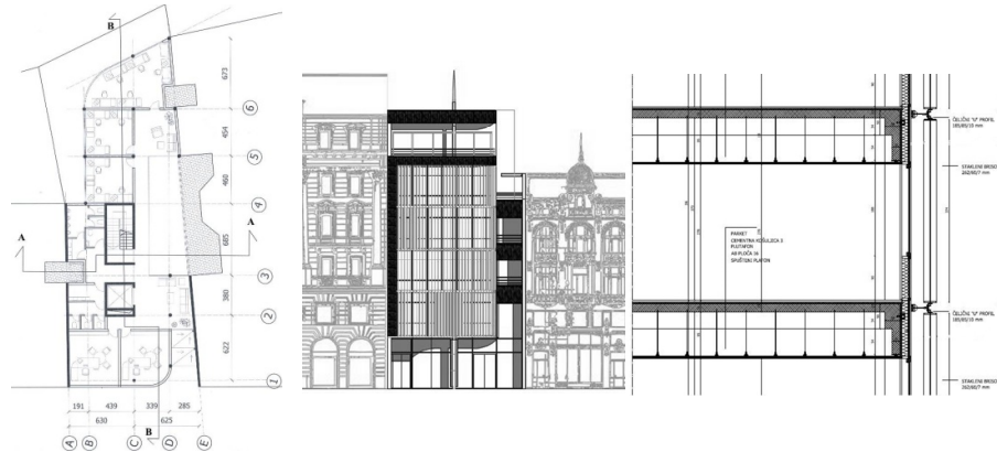
Figure 5. Plan of a typical floor, elevation and cross-section of the street facade of Model 3
