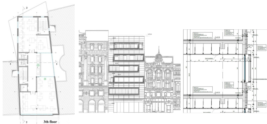
Figure 3. Plan of a typical floor, elevation and cross-section of the street facade of Model 1
