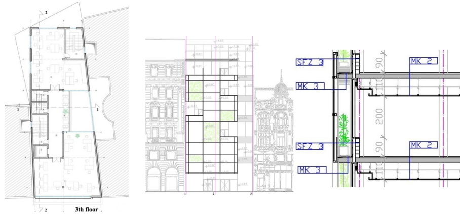
Figure 4. Plan of a typical floor, elevation and cross-section of the street facade of Model 2
