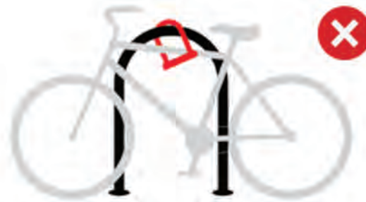
U-Lock secures bicycle frame only, leaving both wheels vulnerable to theft.
