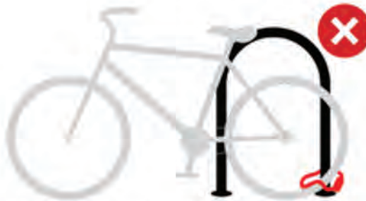
Cable lock secures rear wheel only, leaving rest of bicycle vulnerable to theft.
