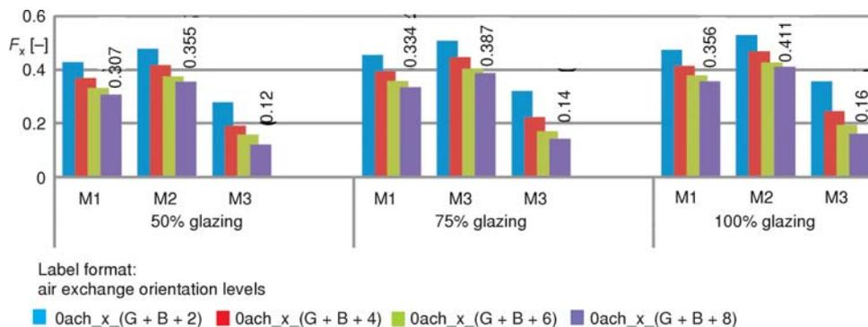
**Figure 5.**  $F_x$  values for three analyzed models with respect to the glazing percentage (stationary temperature mode) (for color image see journal web site)
