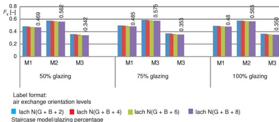
**Figure 6.  $F_x$  values for three analyzed models with respect to the glazing percentage (dynamic temperature mode: 1 exchange per hour and northern orientation)**
