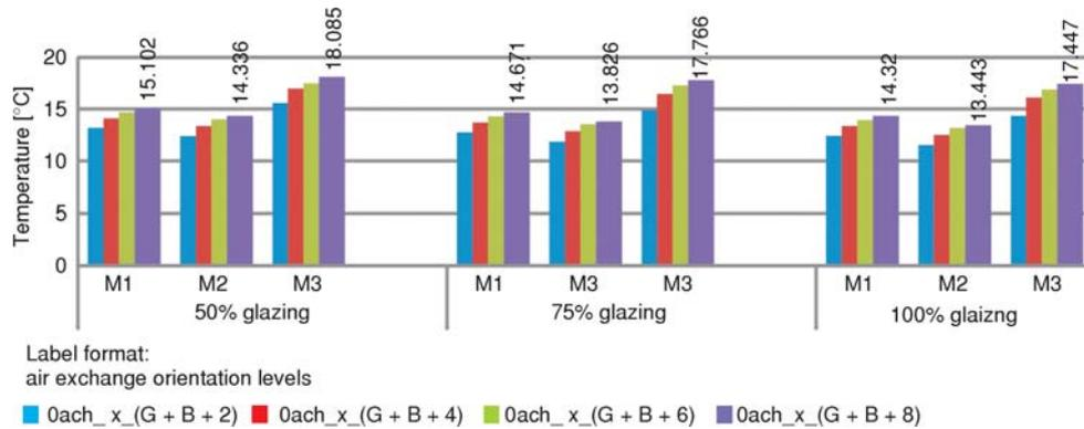
**Figure 4.** Average temperature values for three analyzed models with respect to the glazing percentage (stationary temperature mode) (for color image see journal web site)
