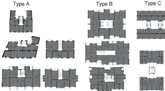
**Figure 1.** Examples of different positions of a staircase within a floor plan of a building
