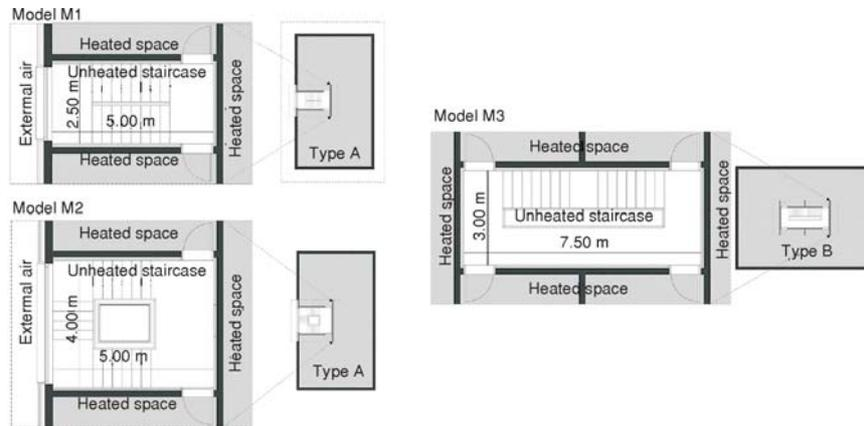
**Figure 2.** Geometry and disposition within a floor plan of model staircases
