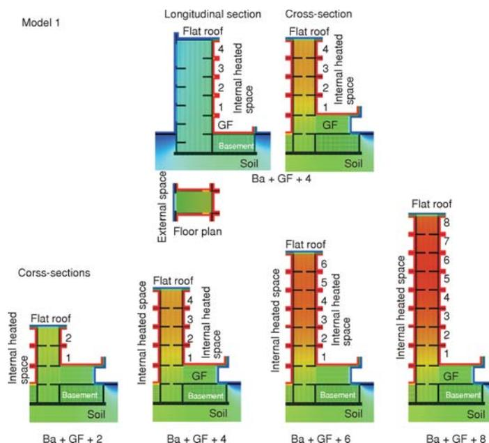
Figure 3. Temperature distribution pattern along the Ba + GF + 4 high model M1 staircase area (top) and variations in temperature distribution due to the change of building height (bottom) (for color image see journal web site)
