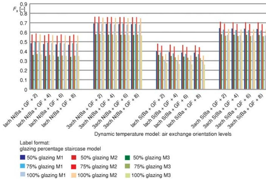
Figure 7.  $F_x$  values for three analyzed models with respect to orientation and air exchange rate (for color image see journal web site)
