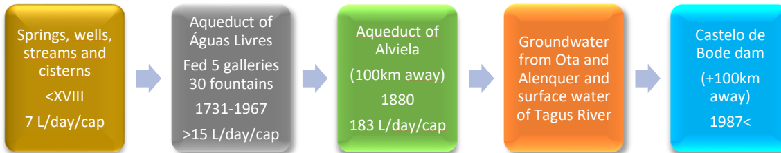
Evolution of the water sources supplying the Lisbon city and the availability of water per capita
