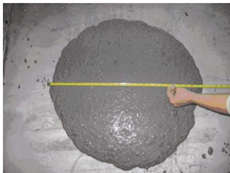
Figure 7: Resulting concrete spread 670 mm (class SF2)
