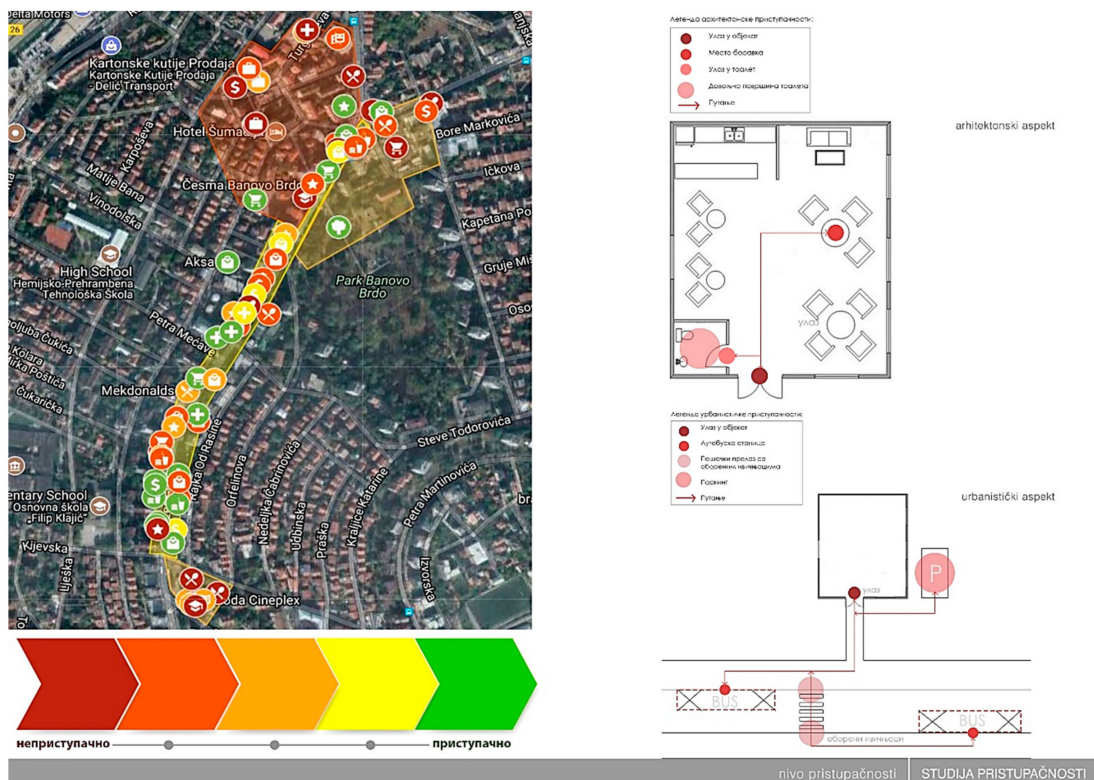
Figure 6. The interface of a submitted application form providing information on the accessibility of possible routes which could be used by the institutions responsible for the implementation and supervision of standards. Left: The accessibility levels of a route (the scale was defined after feedback from the users and the Serbian Alliance of Paraplegics and Quadriplegics). Right: The visualization of the selected spot—architectural and urban accessibility. Source: https://limitless.org.rs/map/ .
