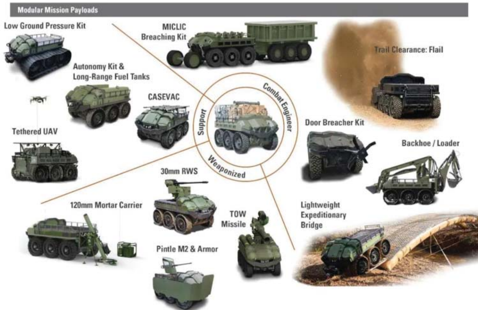
SLIKA 5 _ Različiti modeli besposadnih zemaljskih vozila (izvor: THE DRIVE. THE WAR ZONE. Experimental Marine Unit Deploys 'Hunter Wolf' Unmanned Ground Vehicles For Mountain Training. Preuzeto sa: https://www.thedrive.com/the-war-zone/44200/experimental-marine-deploys-hunter-wolf-unmanned-ground-vehicles-for-mountain-training )
