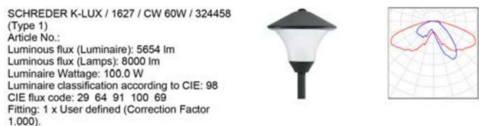
Figure 2. Characteristics of the existing lamp [10]
