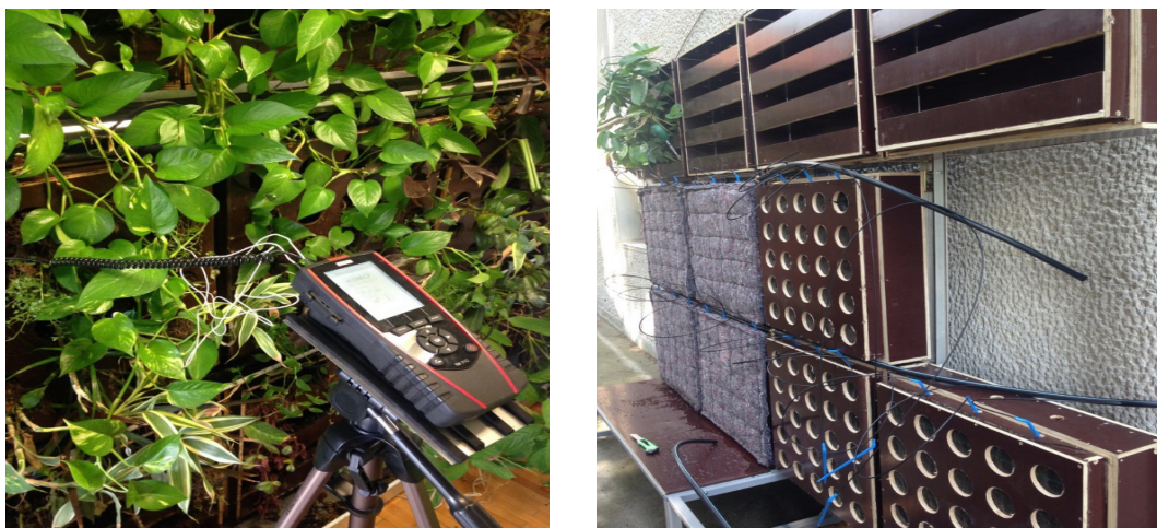
Figure 4. Measurement of contact temperatures by the device Kimo TM 210 (photos taken by authors)
