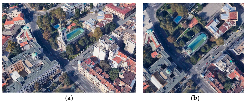
Figure 15. Installation of PV panels on the rooftop of the Cathedral of St. Michael the Archangel in heritage area of Belgrade called Kosančićev venac. (a) 3D view; (b) Top view (Google maps and authors).
