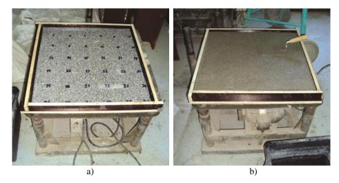
Fig. 2 Manufacturing of the pilot element on a vibrating table: a) mould with placed stone tiles, b) embedding the mortar mixture
