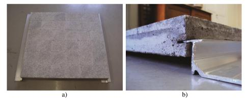
Fig. 3 The manufactured façade panel: a) the pilot element with placed carrier rails Tabaš, b) a detail
