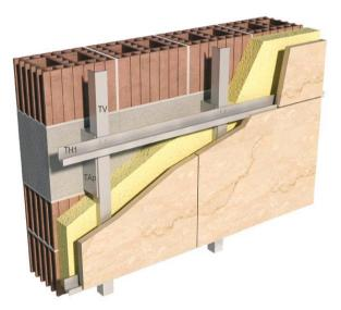
Fig. 6 A ventilated façade carrier system Tabaš [24]
