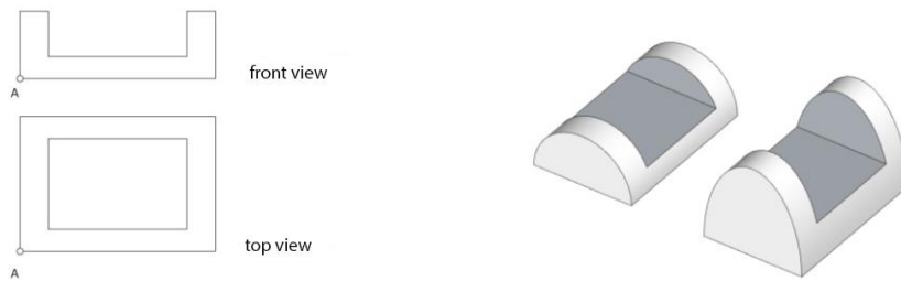
Fig. 2 The text of the task is following: On the left you see top view and front view of certain solid. If there are some hidden lines, they would be presented as dotted lines. Can you imagine and draw what would this solid look like in isometric view? Sketch at least one possible solution. The answer is given on the right. Source: Informer for prospective students of FACEG in Banja Luka
