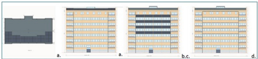
Figure 2: (a) I Design Variant: roof 40° (roof and facade layouts), (b) II Design Variant: parapet 90°, (c) III Design Variant: parapet 45° and (d) IV Design Variant: sun shading 0°
